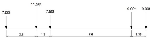
Figure 3. Somerset Bridge. 5 Axle 44 ton vehicle layout.
